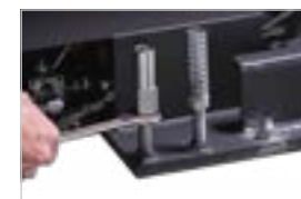
○ Adjusting Screw For Leveling The Base
